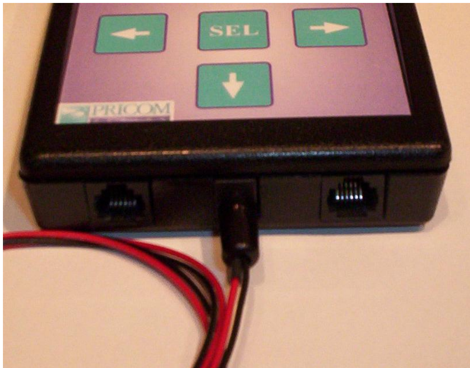
Figure 2 - Track Wire Connection
